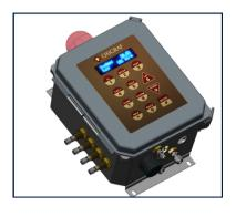
Now optional on the O2iM safety monitor is multiport sampling. Up to four (4) sample locations can be monitored by a single O2iM unit through an internal sample port multiplexer. The O2iM will automatically sample and switch sample input ports and internal valves and fittings are added to the standard housing equipped with the 5-relay board option which contains the required circuitry for this feature.
