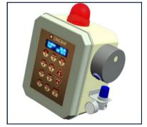
The O2iM unit features a Z-Purge system for use in Class 1 Div 2 hazardous areas, requiring a nitrogen gas source for inerting. It includes a purge indicator and gas regulator with remote status output. Additionally, the OxiPurge option allows for enclosure purging in non-hazardous situations to prevent contamination and maintain dryness, with a VFD display to notify if the purge is lost.
